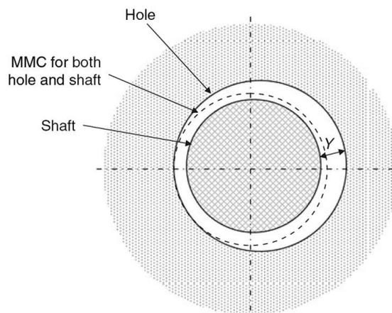
Figure 2: Assembly of hole and shaft sizes
