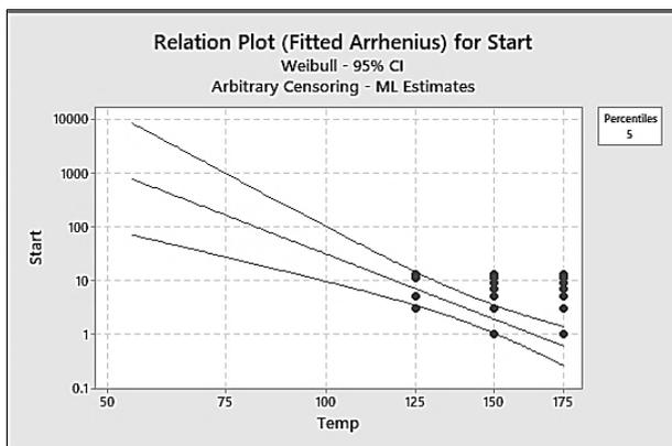
Figure 8: Probability diagram of the start of the Appliance reliability check
