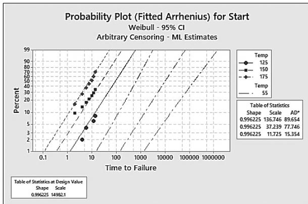
Figure 7: Probability diagram of an accelerated product reliability check
